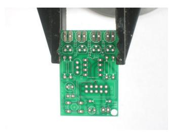
Check the kit against the <u>parts</u> <u>list</u> (http://adafru.it/c5r) to verify you have all the parts necessary.
