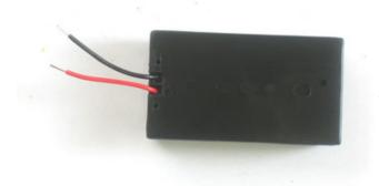
Strip the ends of the wire off so that there's a short section without insulation.
