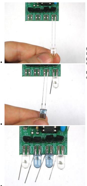
Next is the IR LEDs. Start with **LED1**, a clear IR led. Like the small indicator LED, it has polarity. Make sure the longer, positive lead is on the right, as shown.
