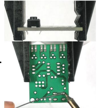
Using your soldering iron, heat up a leg of the button and the poke solder into it to make a nice solder joint.
