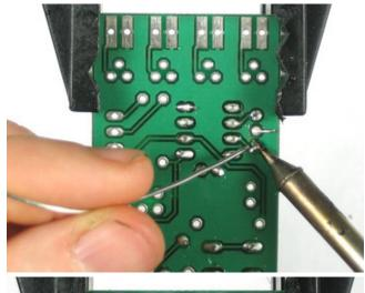
Solder the rest of the points then clip short the legs of the oscillator.
