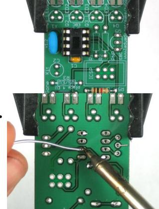
Next, place 2 components. The ceramic oscillator and the 8-pin socket. The oscillator has 3 pins and is symmeteric. The oscillator is the timeclock for the microcontroller, making sure that it is performing its functions at the correct speed.
