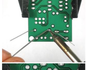
Solder each leg of the resistor.
