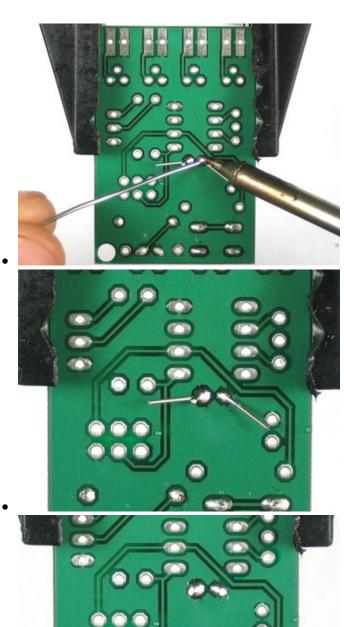
Solder and clip the ceramic capacitor part.
