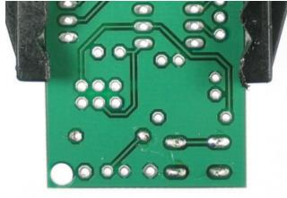
Use the diagonal cutters to clip off the resistor legs so that only the solder points remain.
