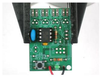
Next place the 1.0K ohm resistors, **R1**. This is the base resistor for the PNP transistor.
